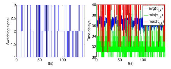
Figure 6. Left: Time-varying switching signal  $\sigma(t) \in \{1, 2, 3\}$  for the communication topology  $\mathcal{A}_{\sigma(t)} \in \{A_1, A_2, A_3\}$  with  $A_i, i = 1, 2, 3$  given in Fig. 5 (Simulation 2). Right: time-varying delays (average value, minimum and maximum) for Simulation 2.
