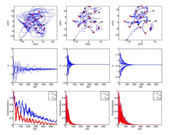
Figure 4. Comparative results between non-predictor (left), proposed weighted predictor (middle), and predictor control (right) given in Table I under time-varying delays  $340 \le \tau_{ji,k} \le 440$  and switching topology  $\mathcal{A}_{\sigma(t)} \in [A_1, A_2, A_3]$  given in Fig. 2 (Simulation 1). First row: trajectories followed by each agent. Second row: Estimation of the angle  $\hat{\phi}_i$ , and Third row: Normalized cost functions  $J_{1,k}$  and  $J_{2,k}$  in (52)
