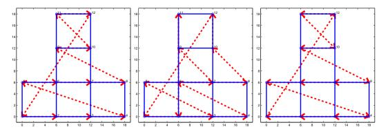
Figure 5. Target formation (solid blue lines) and switching communication topology with lower degree of connectivity (dashed red lines) with  $A_s$ , s = 1, 2, 3 for Simulation 2.
