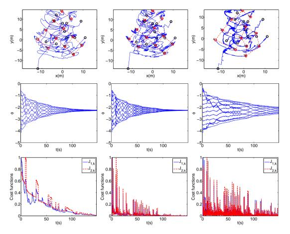
Figure 7. Comparative results between non-predictor (left), proposed weighted predictor (middle), and predictor control (right) given in Table II under time-varying delays  $30 \le \tau_{ji,k} \le 40$  and switching topology  $\mathcal{A}_{\sigma(t)} \in [A_1, A_2, A_3]$  given in Fig. 5 (Simulation 2). First row: trajectories followed by each agent. Second row: Estimation of the angle  $\hat{\phi}_i$ , and Third row: Normalized cost functions  $J_{1,k}$  and  $J_{2,k}$  in (52)
