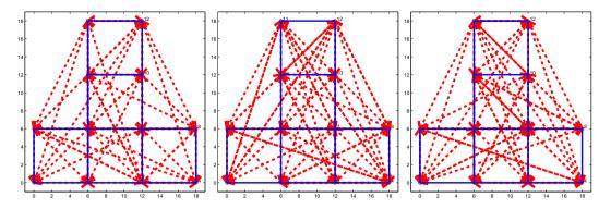
Figure 2. Target formation (solid blue lines) and switching communication topology (dashed red lines) with  $A_s$ , s = 1, 2, 3 for Simulation 1.
